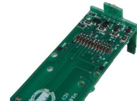
The boards are put together as "H-bridge", and secured by solder from bottom side. The small LED boards are interchangeable. You can swap the boards regardless which side they get mounted.
