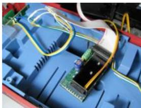
The cabling from Piko has all head lights from motor coach and side car coupled. The connections 7, 10, 14 (counting scheme decoder pin) are not used in this mode. To allow extra switch off of the rear motor coach headlights small soldering work is necessary on the distributor boards at the rear end of the motor coach.
