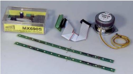
Base component is the ZIMO MX690S sound decoder. The MX69S might be used as well, this is a similar decoder without sound functionality. For coach light the user might use any light board or the AMW Digital LED which provides enhanced functionality.
