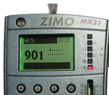
ATTENTION the MX9 monitor does not work on a MX31FU in wireless mode to save bandwidth. It is necessary to operate the MX31FU in cable mode! Use a CAN Bus splitter temporarily to insert the MX31 for diagnostic purposes.
