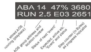
To increase reliability, it is recommended to change the speed a bit after a sync point has been passed. This allows the MX1 to change the speed of the loco at this point. Doing that increases precision of halt points, as timing and speed are resynced to that location. The Exx information in the MX1 display informs which sync line was triggered. The information stays in the display for some seconds.
