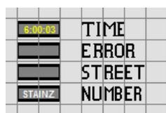
mediately displayed. Keep in mind that only limited space is available in the display field. The loco number is displayed as well for **any** track section in a field on the upper right corner, if the mouse pointer is moved over it. The picture to the left shows this situation. The loco text “STAINZ” is displayed here while the mouse was pointing to a section where loco number 2 was causing an occupation.
