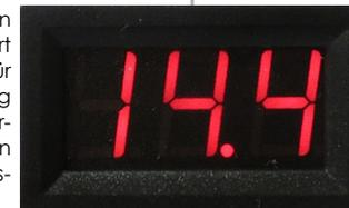
The meter is based on a digital instrument which is combined with 2 signal processing boards. The meter carries some modifications inside to correct the losses of the signal processing boards.
